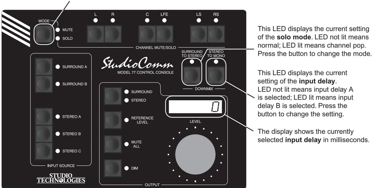
**Figure 11. Solo mode and input delay settings**
