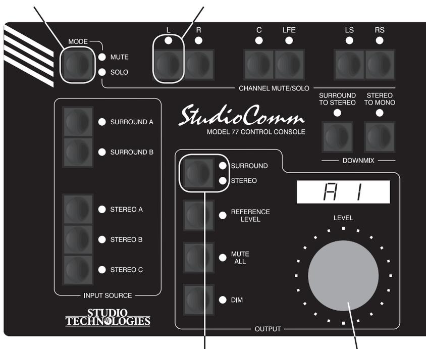
These LEDs display the status of the **post-fader stereo monitor output** function. When LED Surround is lit the function cannot be enabled. When LED Stereo is lit the function can be enabled. Use the button to change the configuration.
