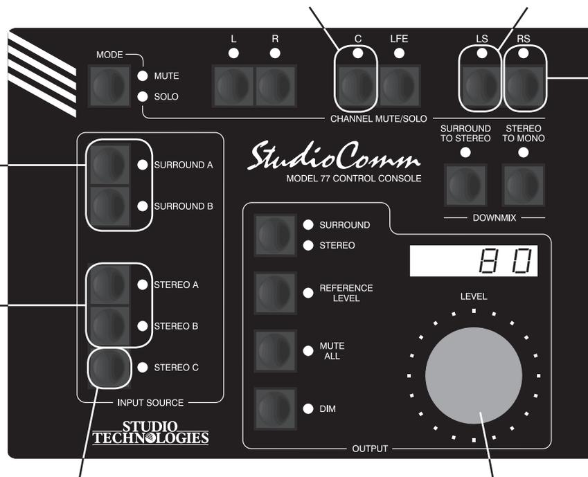
This LED displays the configuration of the **mute/solo bass management mode**. LED lit means mute/solo functions occur post-bass management; LED not lit means mute/solo functions occur pre-bass management. Use the button to change the configuration.
