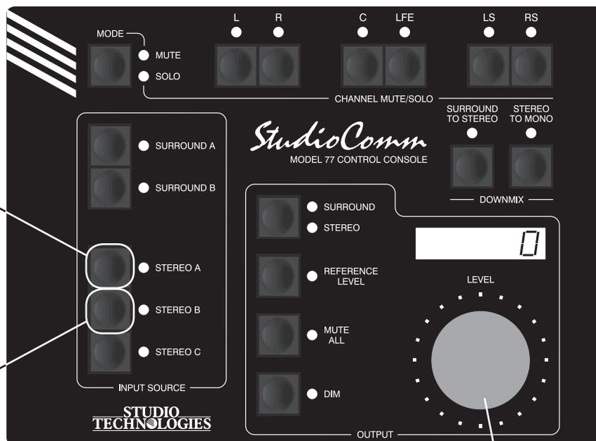
Use the level control to adjust the **input delay**. Range is from 0 to 340. The display shows delay in milliseconds at 48 kHz sampling rate. The value is scaled up or down for other sample rates.
